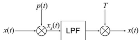
The sampled signal  $x_s(t)$  can be stored in computer memory or in some other digital medium and then later recovered using the interpolating filter.
