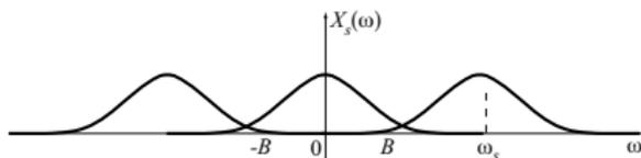
For audio signals, aliasing results in warbling at high frequencies. In image processing, aliasing leads to the so-called *moire effect*, i.e., periodic ringing.
