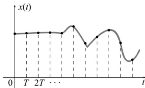
Given the **sampling period**  $T > 0$ , we convert a continuous-time signal  $x(t)$  into a discrete-time signal  $x[n]$ , where
